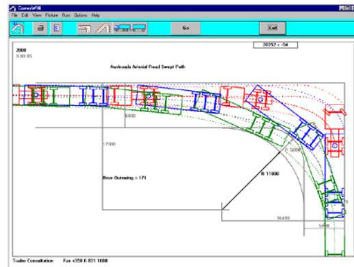
CornerWIN is normally used in conjunction with **TrailerWIN**. The dimensions for the truck and trailer are made in TrailerWIN and this combination will be transferred automatically to CornerWIN.
