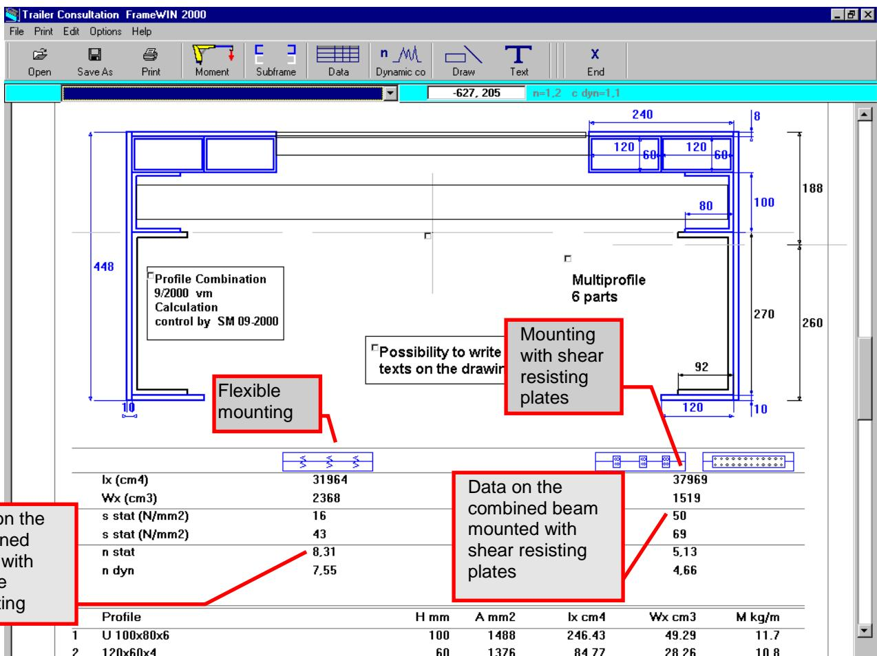
FrameWIN is a software created for subframe calculation and it helps you to choose a suitable subframe-profile when assembling crane and tailgate lifters.
