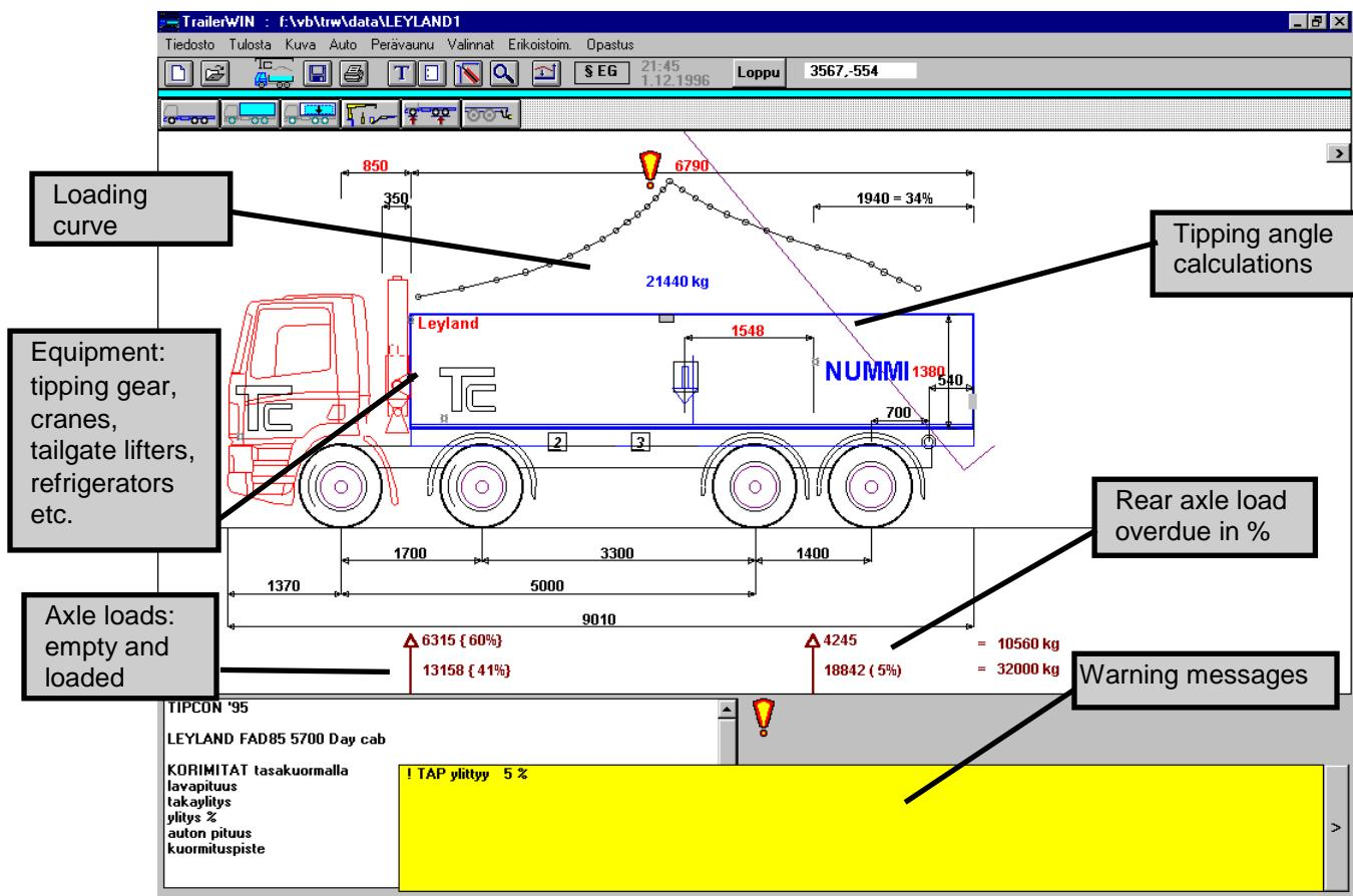
TrailerWIN does the truck body calculations in accordance with weight distribution, total vehicle length, load weight point etc.
